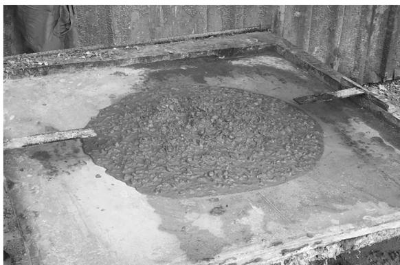
**Figure 2.** Flow test of one of the mixes produced in this project giving evidence on the self-compacting properties of the material
