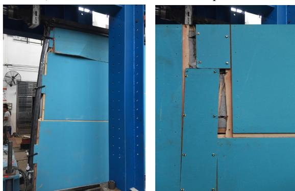
(a) Bending and fracture in the sheathings
