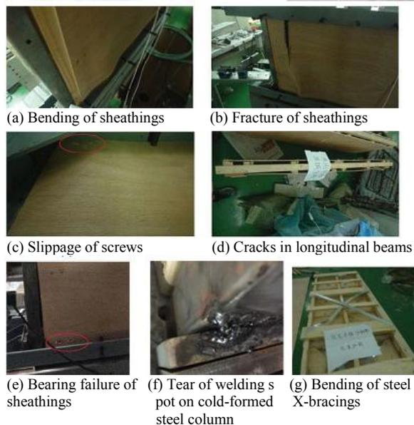
Fig. 7. Failure modes of CTWPs.
