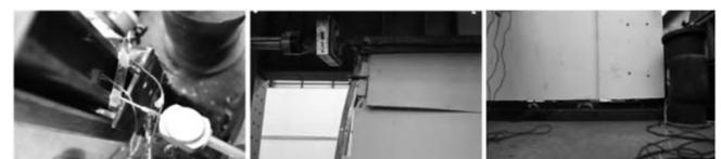
(a) Bending of sheathings (b) CTWP tilting away from the ground frame beam (c) Tear of welding spot cold-formed steel column
