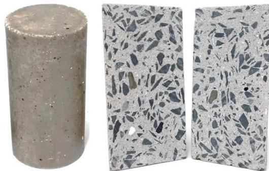
**Fig. 4.** AABC in hardened state and distribution of aggregates.
