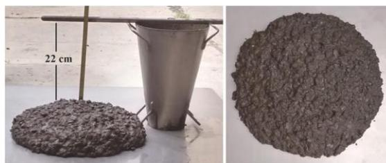
**Fig. 3.** Slump and appearance in fresh state of the AABC.
