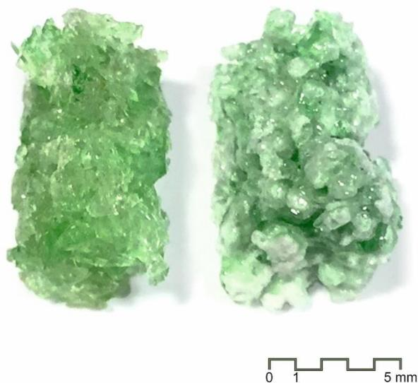
**Fig. 2.** Macro photography of samples compacted with geopolymers (left), and thermally at 700 °C (right). Note the rounding of aggregates of glass after heat treatment (right) and its better compaction.
