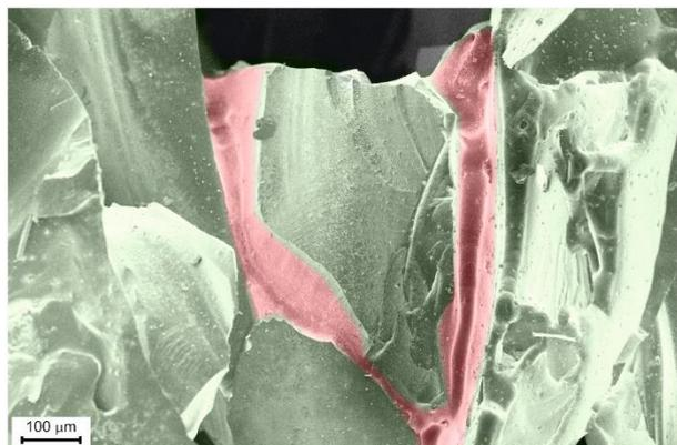
**Fig. 5.** SEM detail of the "mortar" made of glass aggregates and water glass binder. Note the sharp edges of the aggregates (green). The binder filled the pores and fissures (red color).
