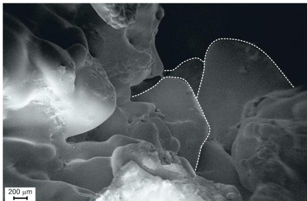
**Fig. 8.** Detail of sample compacted at 700 °C/12 h. Rounded grains (dotted line in white color) partially melted are highlighted. Water glass binder is also melted, filling pores and cracks.
