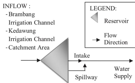
Fig. 2. Gunungrowo Reservoir system schematic
