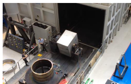
Fig. 1. Open vacuum chamber of the pro-beam® EBW facility K2000 showing a welded mock up of a pressure vessel (front)
