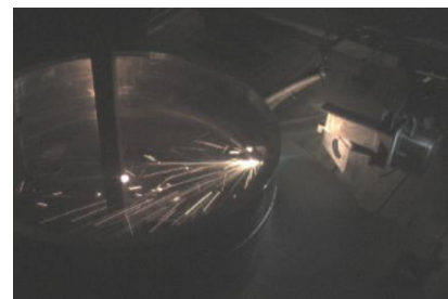
Fig. 5 Circumferential EBW of a shell
