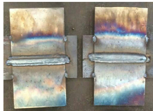
Fig. 2. SM570-TMC steel plates after welding
