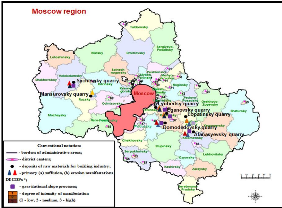
Fig. 5. Schematic map of the spread of surface manifestations of dangerous exogenous geodynamic processes in the quarries for the extraction of raw materials for building industry in the Moscow region.
