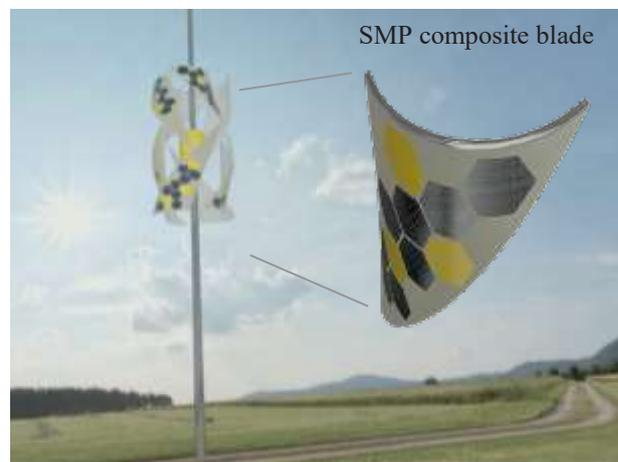
Figure 11. Small wind turbine with SMP composite blades.
