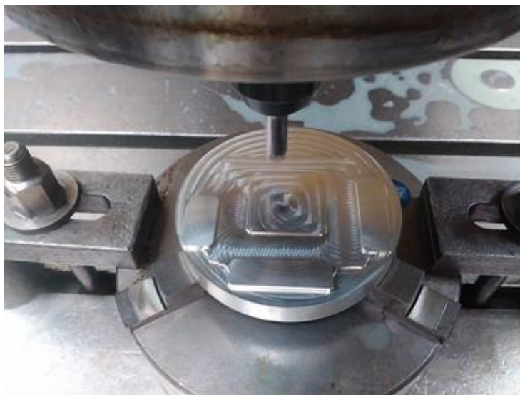
Fig. 9. Machining thin-walled component on the vertical CNC milling centre Pinnacle 2100.
