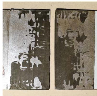
**Fig. 5.** Photograph of specimen #A after separation.
