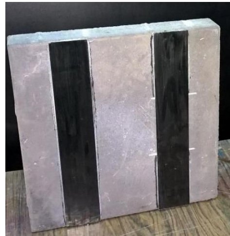
Fig. 7. Specimen of CFRP strips for initial thrmography tests
