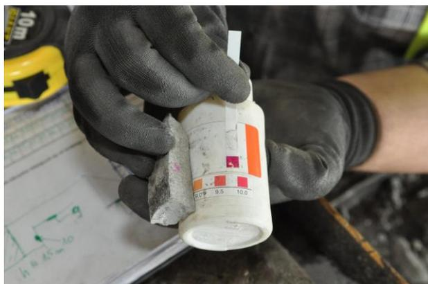
**Fig. 1.** Concrete sample tested after 50 years of service life.
