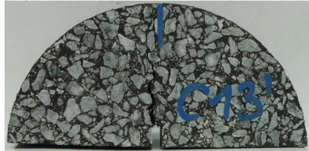
**Fig. 3.** Stone matrix asphalt SMA 8
