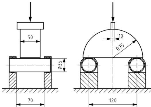
**Fig. 1.** Semi-circular test specimens subjected to three-point bending
