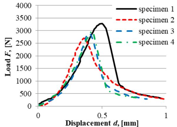
**Fig. 6.** Laboratory test results for notch depth 20 mm, PA 8
