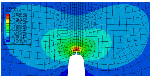
**Fig. 11.** Cohesive element crack model - propagation of crack
