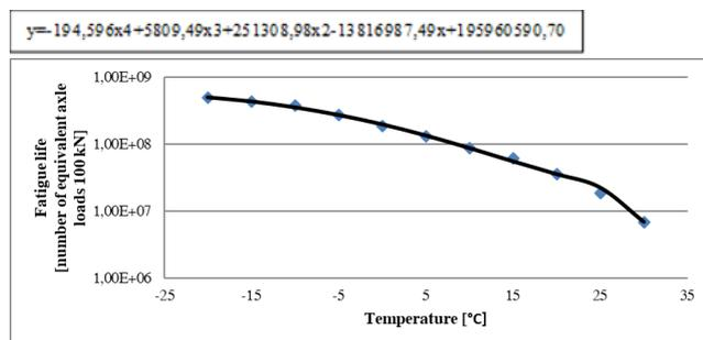
**Fig. 6.** The resulting fatigue curve from the calculations with use of AASHTO 2004 criterion
