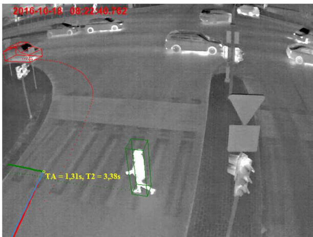
Fig. 4. T-Analyst – identification of vehicle/VRU trajectories and assessment of conflict severity by automatic calculation of various surrogate safety indicators.
