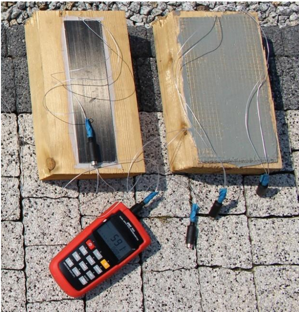
Fig. 1. Test of the influence of solar radiation o temperature.
