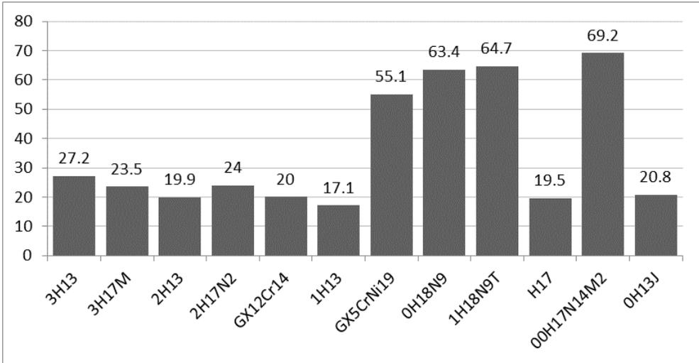
**Fig. 1.** Comparison of environmental indicators (in mPt) for selected steel and cast steel gearwheels
