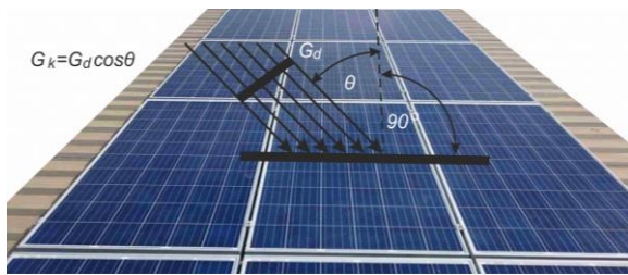
Fig. 5. Influence of the angle of incidence \theta of solar rays with the intensity G_d on the surface of the modules on the value of radiation intensity G_k .
