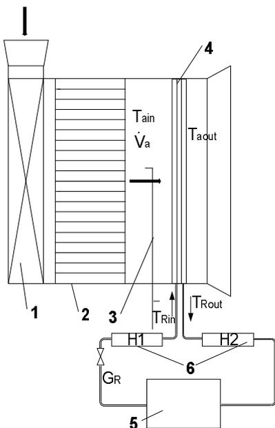
**Fig. 2.** Experimental setup: 1-radial fan, 2-flow stream equalizer, 3- Pitot tube, 4-studied tubes, 5-condensing unit, 6-electric heaters.
