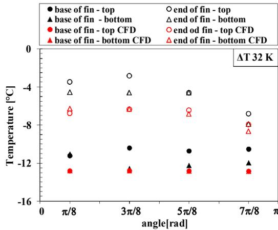
**Fig. 8.** Temperature distribution for CFD calculations, for mixed convection,  $\Delta T=32K$ ,  $w_a=2.3$  m/s.
