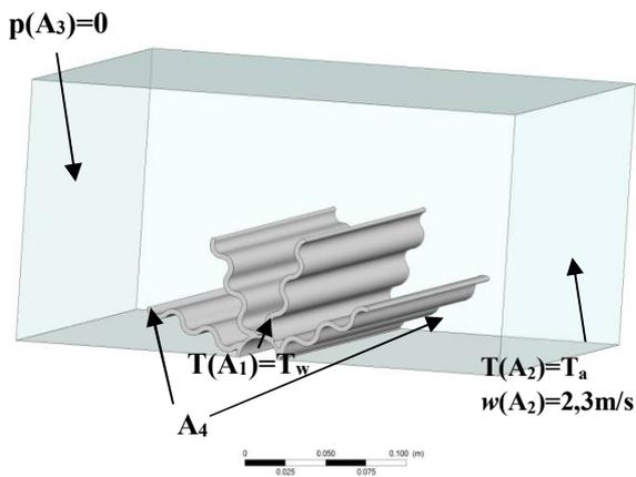
**Fig. 5.** The model and the boundary conditions.
