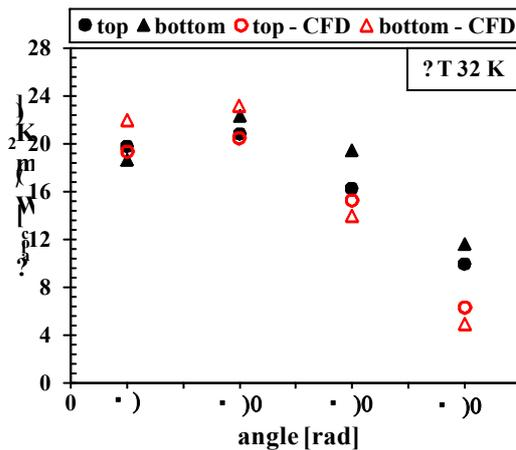
**Fig. 9.** Example of local heat transfer coefficient values obtained from CFD modeling for mixed convection,  $\Delta T=32K$ ,  $w_a=2.3$  m/s.
