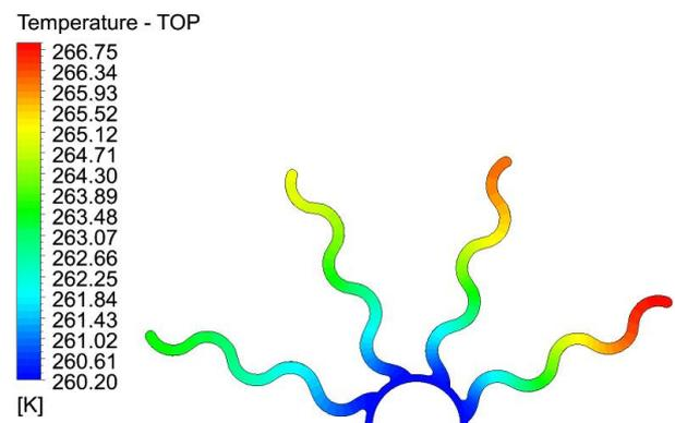
**Fig. 6.** Temperature distribution for CFD calculations, for mixed convection,  $\Delta T=32$ K,  $w_a=2.3$  m/s – top of the fin.
