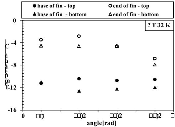
**Fig. 3.** Example of temperature distributions for mixed convection,  $\Delta T=32K$ ,  $w_a=2.3$  m/s.
