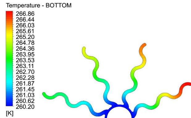
**Fig. 7.** Temperature distribution for CFD calculations, for mixed convection,  $\Delta T=32$ K,  $w_a=2.3$  m/s – bottom of the fin.
