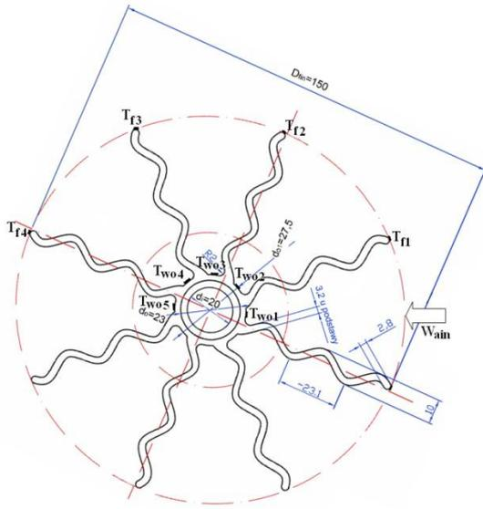
**Fig. 1.** Bimetallic tube cross-section.
