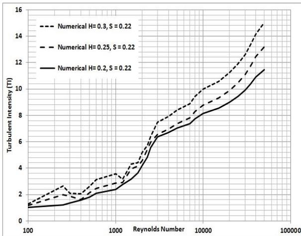
**Fig. 6.** Variation of turbulent intensity (TI) with Re.
