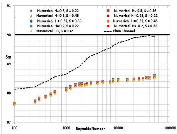
**Fig. 8.** Variation of average synergy angle with Reynolds number for different length and pitch ratio.
