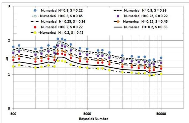
**Fig. 7.** Thermal enhancement factor.
