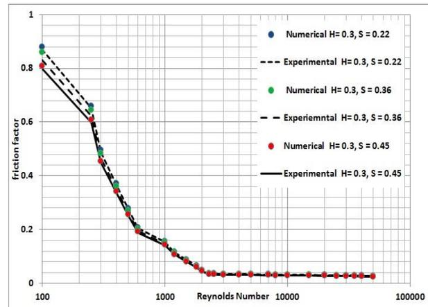
**Fig. 5.** Friction factor as function of Reynolds number, (a) at constant value of length ratio ( $H = 0.3$ ) with different pitch ratio ( $S = 0.22, 0.36, 0.45$ ).
