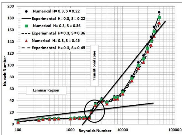
**Fig. 4.** Nusselt number as function of Reynolds number, (a) at constant value of length ratio ( $H = 0.3$ ) with different pitch ratio ( $S = 0.22, 0.36, 0.45$ ).
