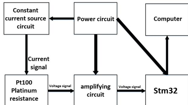
**Figure 4.** Temperature measurement circuit block diagram
