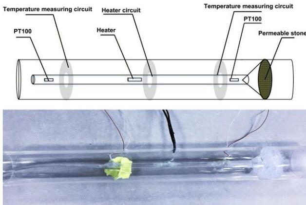
**Figure 1.** Seepage sensor design
