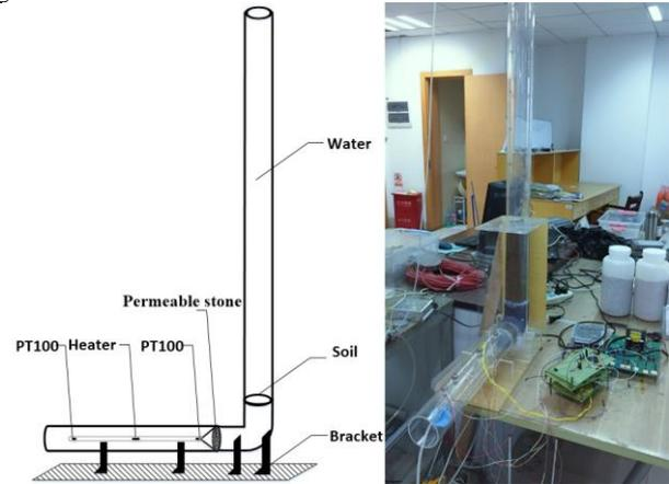
**Figure 6.** Seepage meter calibration experiment device
