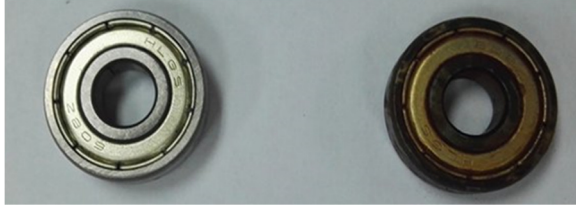
Fig. 1. Particular study case in this paper: Normal bearing (left) and damage bearing (right) due to corrosion.
