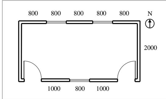
**Figure 2.** Model building with dimensions in mm
