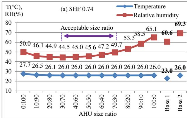
**Figure 3.** AHU acceptable size ratio
