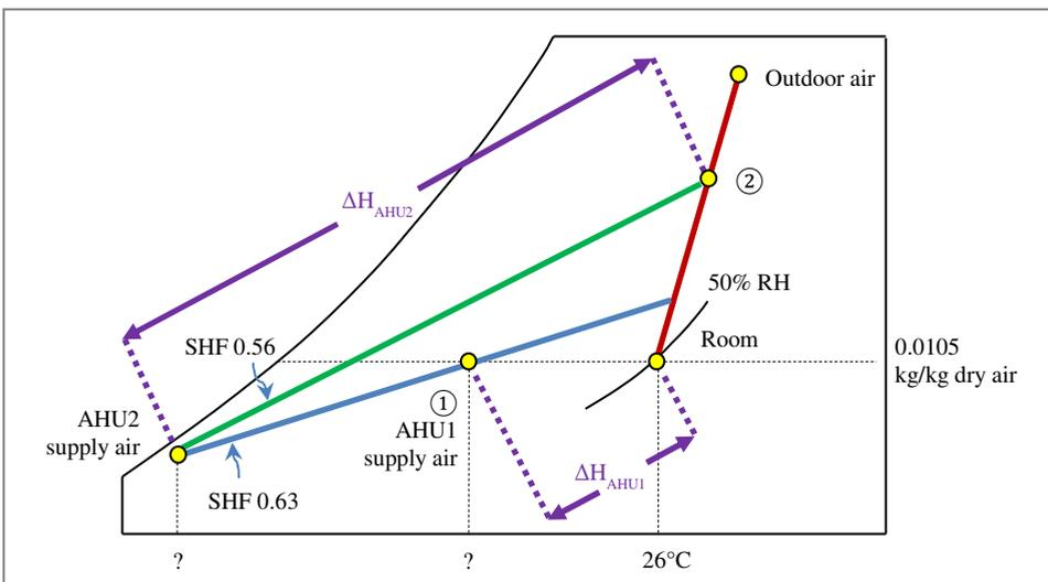
**Figure 4.** Determination of supply air temperature using psychrometric chart
