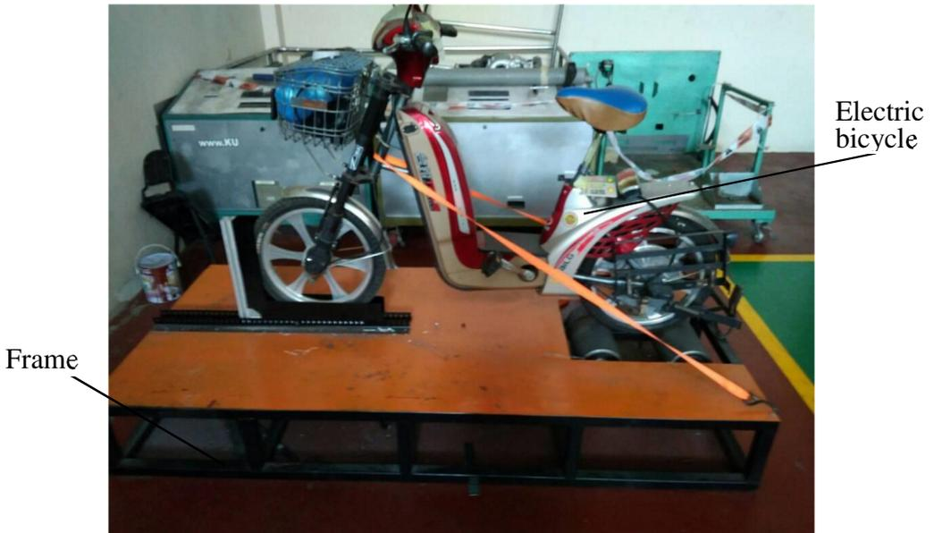
**Fig. 3.** The prototype of chassis dynamometer
