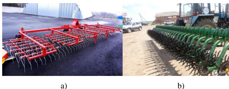
Fig. 1. Modern complex of machines for crop harrowing: a) striegel; b) hinged rotary hoe.
