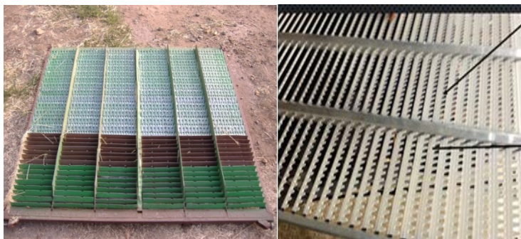
Fig. 2. Experimental combined sieve made of polymer materials.
