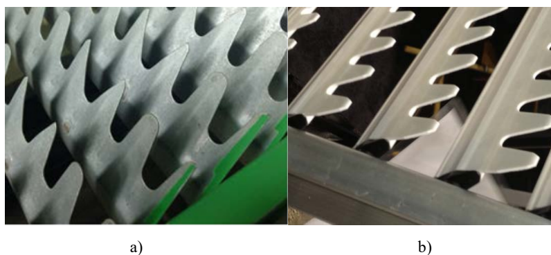
Fig. 4. Type of louvre sieves cleaning the combine harvester a) - metallic, b) - polymer material UHMWPE.
