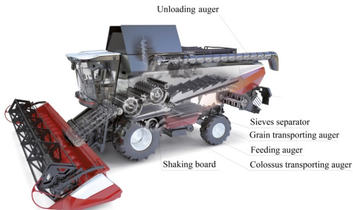
Fig. 1. Complex of working bodies of polymeric materials in the structure harvester combine.
