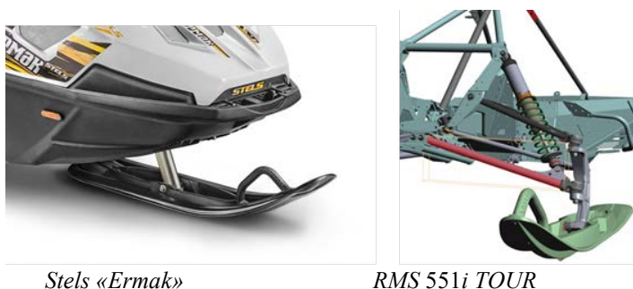
Fig. 10. Front telescopic and lever suspension of snowmobiles Stels "Ermak" and RMS 551i TOUR
