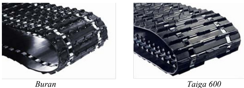
Fig. 8. Caterpillars with gearing through windows and spindle gearing for snowmobiles Buran and Taiga 600
