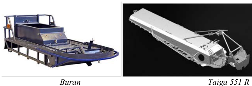
Fig. 3. Platforms for two-track and single-track snowmobiles " Buran " and " Taiga "
