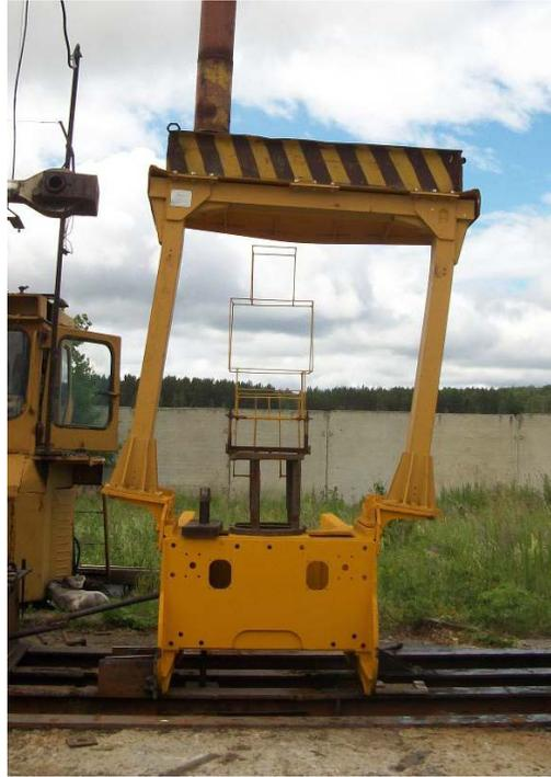
**Fig. 3.** Vertical loading of ROPS
