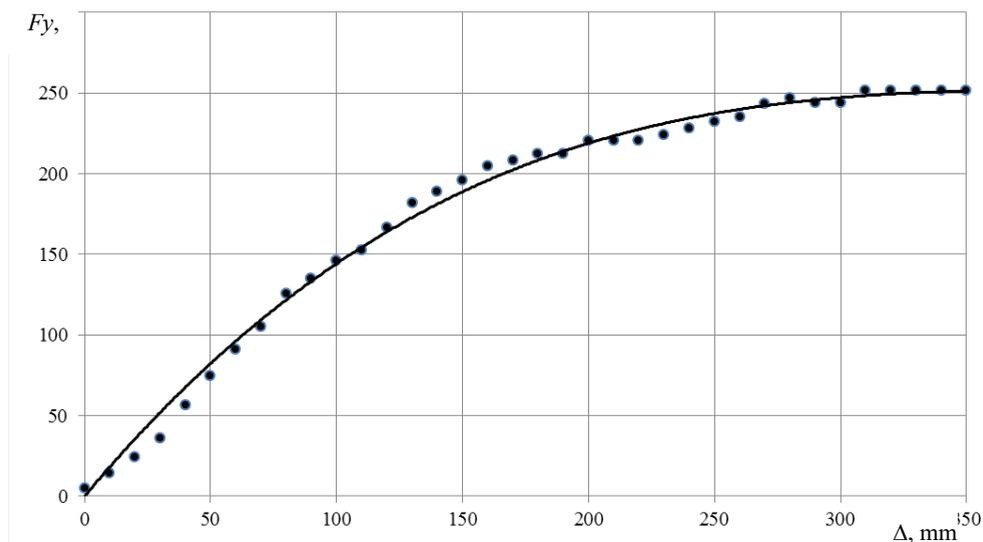
**Fig. 5.** Correlation between the lateral force  $F_y$  and deflection  $\Delta$  of ROPS structure
