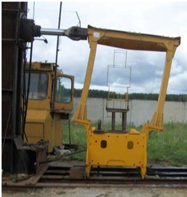
**Fig. 2.** Lateral loading of ROPS
