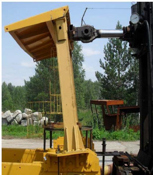
**Fig. 4.** Longitudinal loading of ROPS
