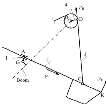
**Fig. 1.** Schematics of the operational equipment mechanism: 1, 4 – cranks; 2 – stick with bucket; 3 – hoisting rope;  $V_H, V_T, V_E$  – velocities of hoisting, thrusting and excavation
