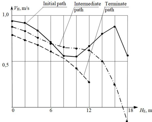
**Fig. 2.** Graphs relating the hoisting velocity to the excavation height for a bucket moving along equidistant paths (excavation velocity  $V_E = 1$  m/s)
