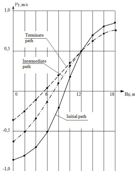
**Fig. 3.** Graphs relating the thrusting velocity to the excavation height for a bucket moving along equidistant paths (excavation velocity  $V_E = 1$  m/s)
