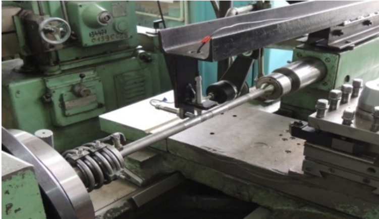
Fig. 3. Experimental machine for turning with a spring driving dog
