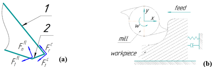
Fig. 1. (a) - the forces affecting the cutting edge; (b) - the model of the compliant technological system.
