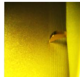
Figure 3. Contact pin under contact with the Leadframe
