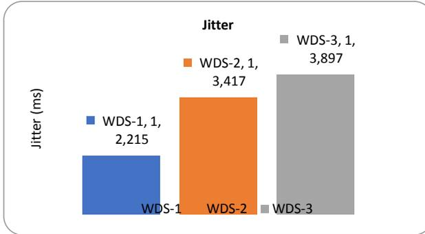
Fig. 6. The comparison result of jitter average value
