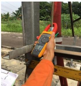
**Fig. 6.** Monitoring leaked Current on the operation
