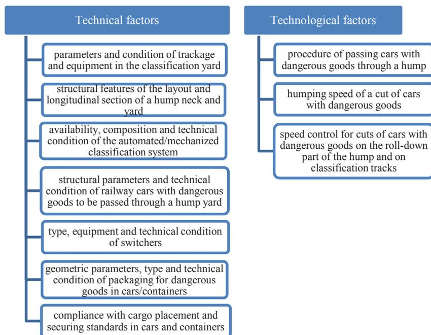
**Fig. 2.** Classification of technical and technological factors that determine the safe conditions for the transportation of dangerous goods.
