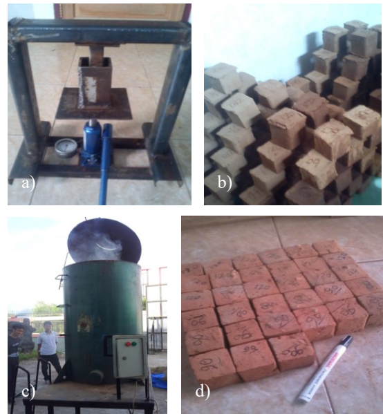
Fig 1. the manufacturing process of the test sample: a) mold, b) green body, c) the burning process, d) sample test
