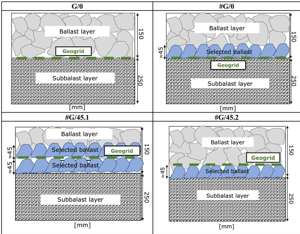
Based on the first model (G/0), the maximum size of the particles that were interlocked was around 50mm. Therefore, the ballast selected for a better interlocking had a maximum size of 45mm. This ballast was selected from the standardized one, using a 45mm sieve.
