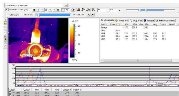
**Fig. 7.** Illustration of thermographic methodology for investigating the process of abrasive cutting.
