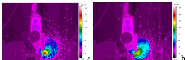
**Fig. 4.** Successive thermograms of the workpiece during the process of cutting
