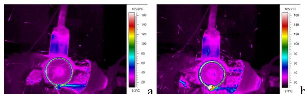
**Fig. 3.** Consecutive thermograms of the cutting disk in the process of cutting
