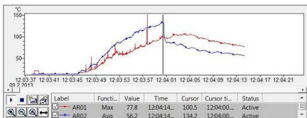
**Fig. 5.** Change of the average surface temperature of the workpiece and the maximum temperature of the cutting surface of the disk before, during and after completion of the cutting
