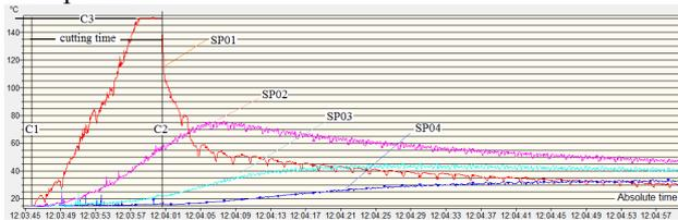
**Fig. 6.** Distribution of the surface temperature of the cut-off wheel, and individual points on the surface of the workpiece measured along the direction of the cutting (SP01 - profile of a point of the cutting disk at  $3 \text{ mm}$  from the periphery; SP02, SP03 and SP04 - profiles of points on the surface of the workpiece located on the distance of  $3 \text{ mm}$  to one another).
