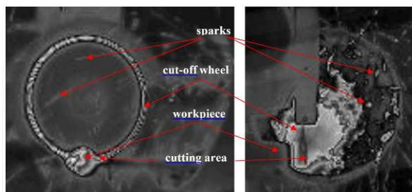
**Fig. 8.** Thermograms after morphological processing
