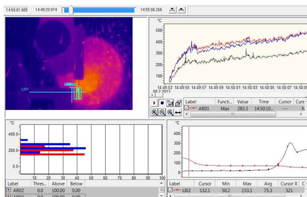
**Fig. 2.** Screen layout with results of thermographic measurements in real time
