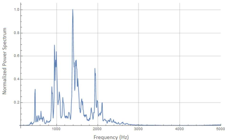
**Fig. 1.** Typical energy spectrum of engine noise. The crankshaft frequency is 20 Hz (1200 RPM).
