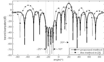
a Transmit beampatterns with 16 transmit array elements
