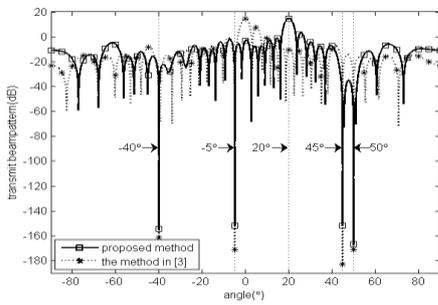
b Transmit beampatterns with 32 transmit array elements
