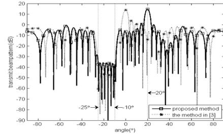
b Transmit beampatterns with 32 transmit array elements
