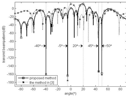
a Transmit beampatterns with 16 transmit array elements
