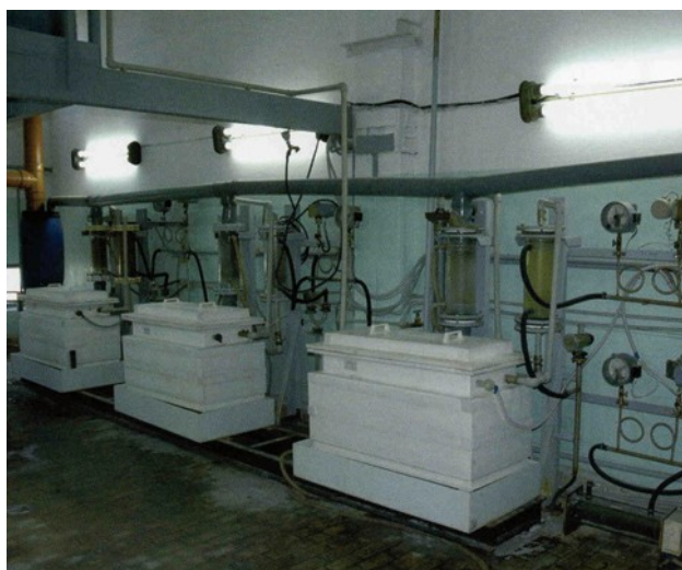
Figure 2. Photo of first generation of the horizontal electrochemical modules for recycling PGM.
