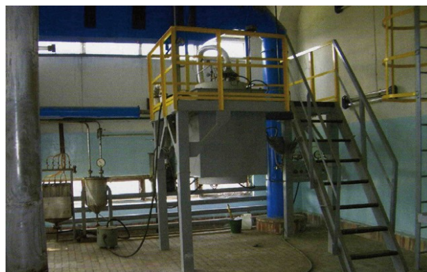
Figure 1. Photo of the furnace for activation of PGM by thermal stabilization of spent catalyst carrier.
