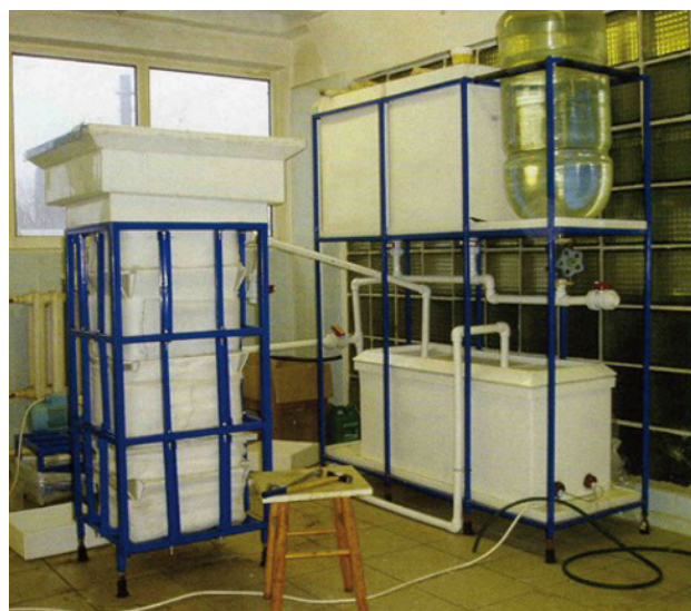
Figure 3. Photo of first generation of the vertical electrochemical module for recycling PGM.
