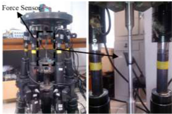
Figure 9. Tensile tests on the MLD.
