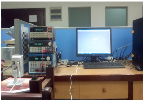
Figure 4. The experimental environment of DMM measurement uncertainty evaluation
