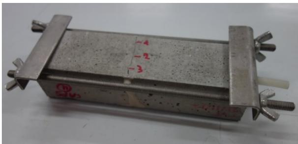
**Fig. 3.** Typical sample for which the crack width is controlled using the CFRP technique.
