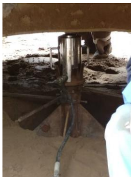
Fig. 5. 3000 cm 2 test plate, supported by an excavator shovel bucket to ensure the specified pressure under the plate
