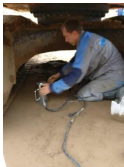
Fig. 5. 3000 cm 2 test plate, supported by an excavator shovel bucket to ensure the specified pressure under the plate
