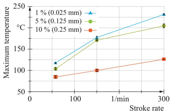
**Fig. 4.** Maximum temperatures occurring during embossing with clearances of 1 %, 5 % and 10 % over stroke rate
