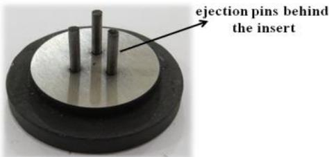
**Fig. 7.** conventional ejection by three pins
