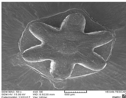
**Fig. 9.** eliminating the curvature of micro gear top surface by hard stopper
