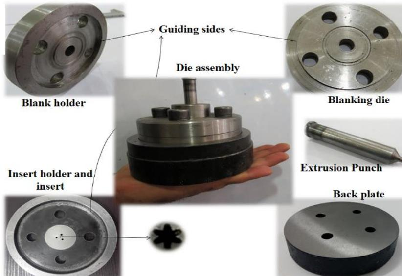
extrusion. Schematic of punches are shown in Fig. 4. The die assembly and components of die are shown in Fig. 5.
