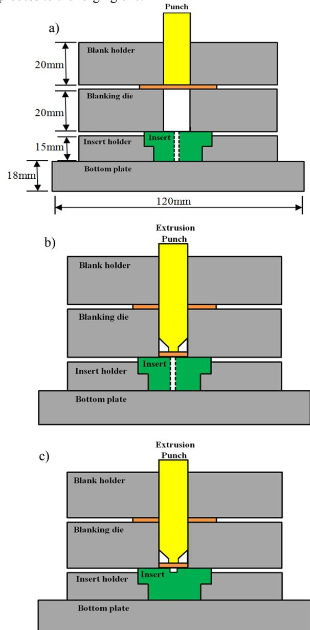
**Fig. 2.** Schematic of the die and experimental procedure
