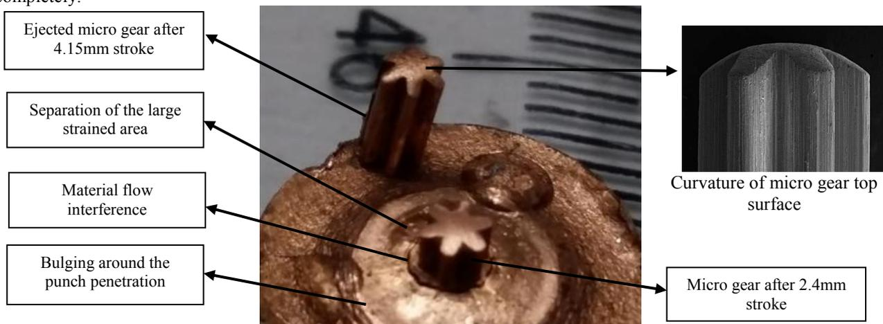
**Fig. 8.** Micro gear formed by single extrusion process at 2.4mm and 4.15mm stroke
