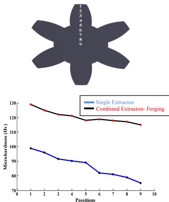
Fig. 10. Micro-hardness – position curve on the cross section of micro gears
