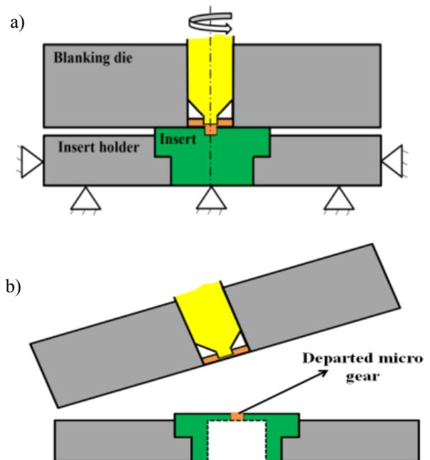
**Fig. 6.** Torsion operation a) keep constant of lower die and twisting of upper die b) picking up the upper die
