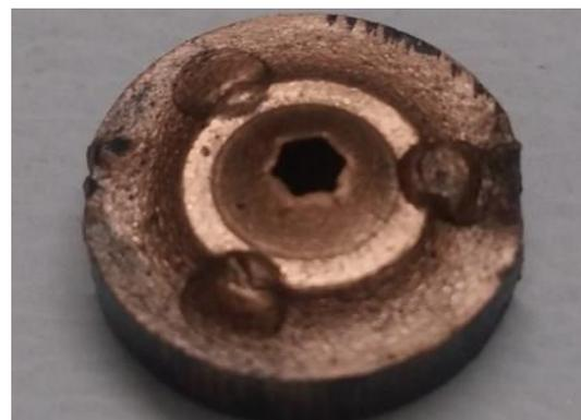
**Fig. 10.** inscribed Hexagon on the teeth and secondary bulging after 4.15mm stroke
