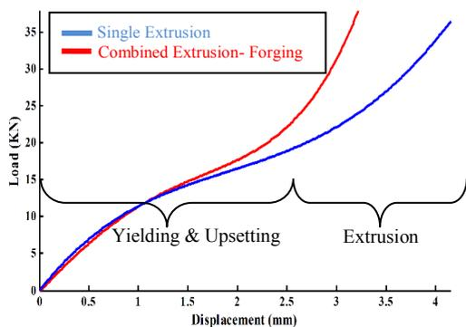
Fig. 9. Load-displacement curve of the micro gears
