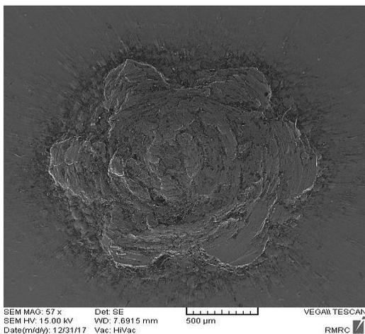
**Fig. 11.** Topography of blank surface after torsion operation
