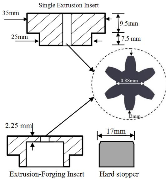
**Fig. 3.** Inserts a) Single extrusion b) Combined Extrusion-Forging
