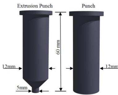
**Fig. 4.** Schematic and size of punches
