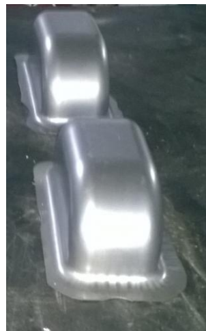
Fig.10. The formed fairing fabricated by hot stamping
