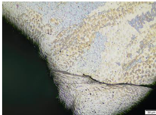
Fig. 7. Crack propagation throughout the oriented dendritic structure within the weld metal.
